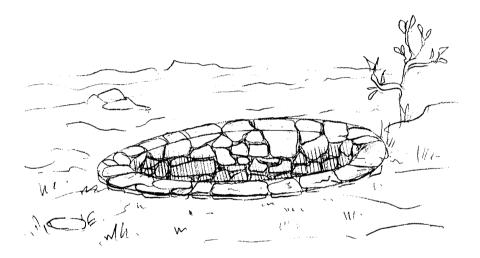
Figure 23: A round-shape sub-surface tank made of stone
