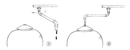
Figure 26: Manual method for separating first-flush
