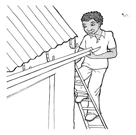
Figure 4: Connecting a gutter system
