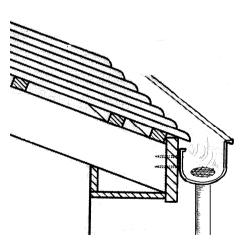
Figure 25: Coarse filter
