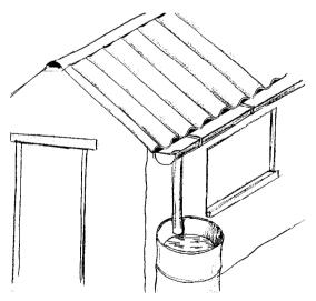
Figure 1: Rainwater harvesting system
