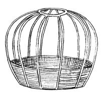
Figure 18: Construction of a water jar with a frame of iron bars or bamboo sticks
