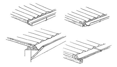
Figure 11: Different types of gutters: square, rounded, V-shaped
