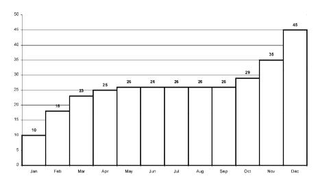
Figure 15: Cumulative monthly roof run-off
