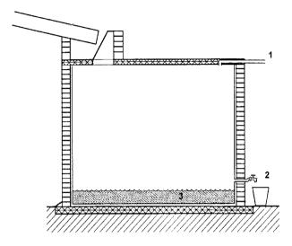
Figure 17: Overflow (1), Tap device (2), Dead storage (3)
