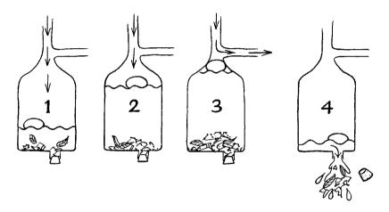
Figure 28: SafeRain system for separating first-flush
