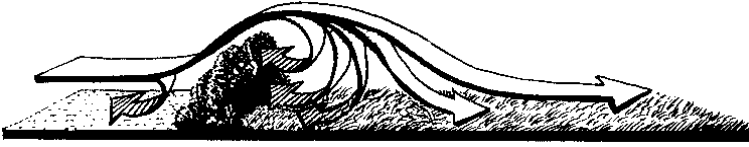
Figure 13: When the shelterbelt blocks the wind completely, turbulence will occur behind the trees and damage the crops.
