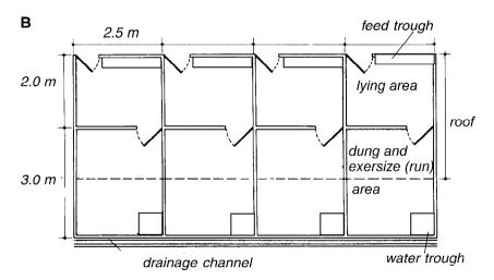
Figure 7: Pen and run for all types of pigs (A: side view; B: top view)
