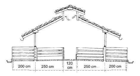
Figure 5: Cross section of a pig house
