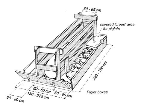
Figure 8: Farrowing crate with covered 'creep' area for piglets
